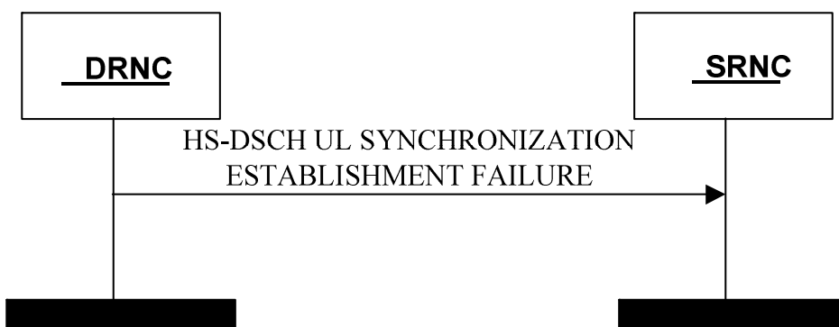
Figure 4AC: HS-DSCH UL Synchronization Establishment Failure procedure
