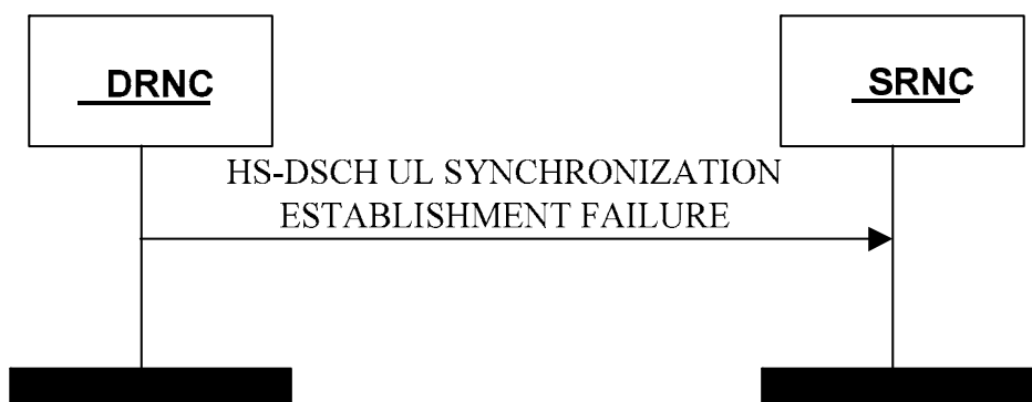
Figure 4AC: HS-DSCH UL Synchronization Establishment Failure procedure
