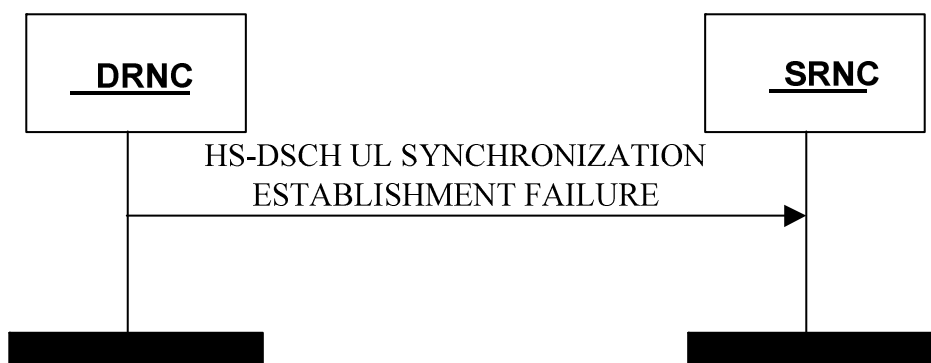
Figure 4AC: HS-DSCH UL Synchronization Establishment Failure procedure
