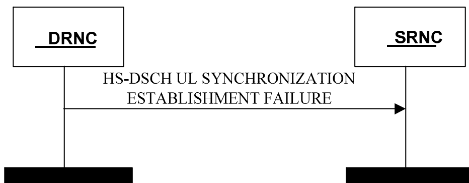
Figure 4AC: HS-DSCH UL Synchronization Establishment Failure procedure
