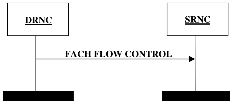
Figure 4A: FACH Flow Control procedure
