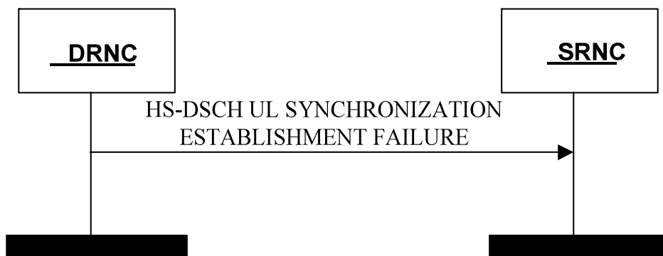
Figure 4AC: HS-DSCH UL Synchronization Establishment Failure procedure
