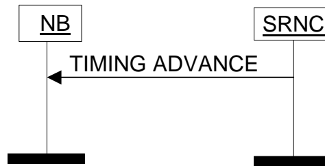
Figure 9A: Timing Advance procedure
