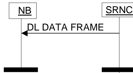
Figure 2: Downlink Data Transfer procedure
