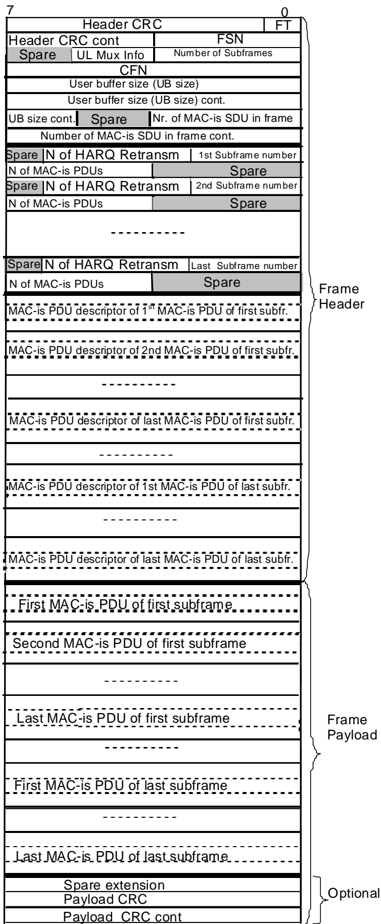
Figure 11b: E-DCH UL DATA FRAME TYPE 2 structure
