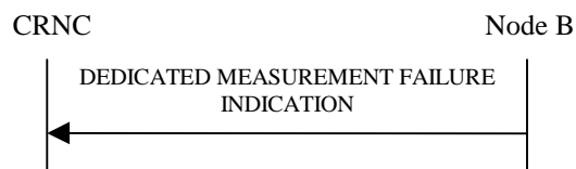
Figure 30: Measurement Failure procedure: Successful Operation
