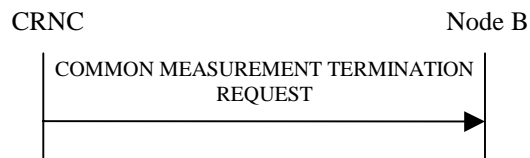
Figure 14: Measurement Termination procedure: Successful Operation
