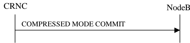
Figure 35: Compressed Mode Commit procedure, Successful Operation
