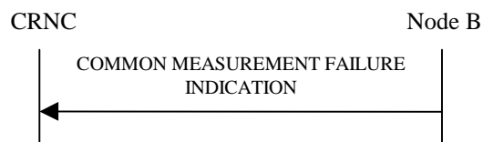
Figure 15: Measurement Failure procedure: Successful Operation
