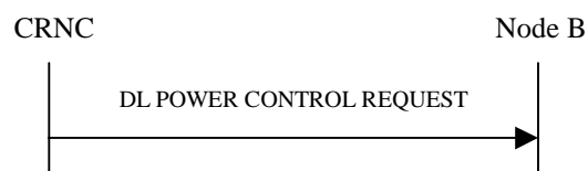
Figure 25: DL Power Control Procedure
