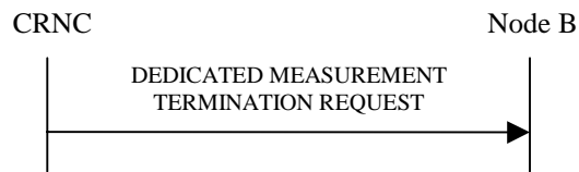
Figure 29: Measurement Termination procedure: Successful Operation
