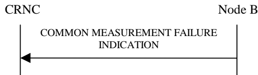
Figure 15: Common Measurement Failure procedure: Successful Operation
