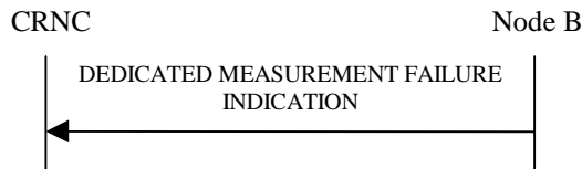
Figure 42: Dedicated Measurement Failure procedure: Successful Operation
