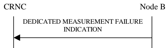
Figure 42: Dedicated Measurement Failure procedure: Successful Operation
