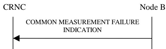
Figure 15: Common Measurement Failure procedure: Successful Operation
