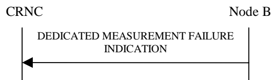
Figure 42: Dedicated Measurement Failure procedure, Successful Operation
