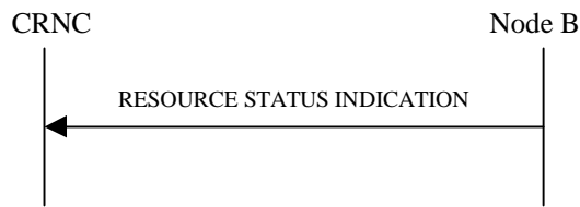
Figure 21: Resource Status Indication procedure, Successful Operation
