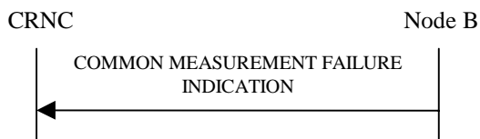
Figure 15: Common Measurement Failure procedure, Successful Operation
