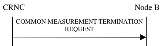
Figure 14: Common Measurement Termination procedure, Successful Operation
