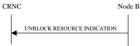
Figure 8: Unblock Resource procedure, Successful Operation
