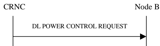
Figure 37: Downlink Power Control procedure, Successful Operation
