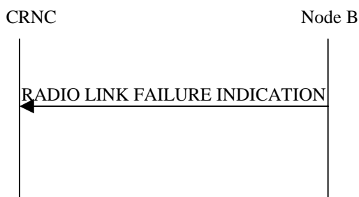
Figure 43: Radio Link Failure procedure, Successful Operation
