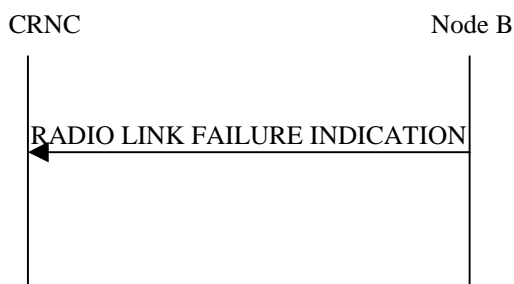
Figure 43: Radio Link Failure procedure, Successful Operation
