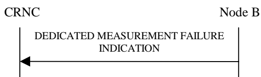
Figure 42: Dedicated Measurement Failure procedure, Successful Operation
