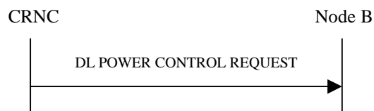
Figure 37: Downlink Power Control procedure, Successful Operation
