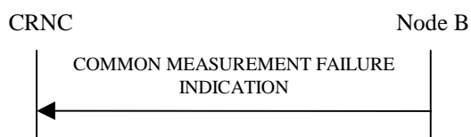
Figure 15: Common Measurement Failure procedure, Successful Operation
