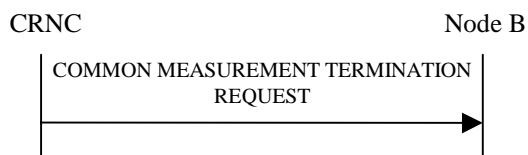
Figure 14: Common Measurement Termination procedure, Successful Operation
