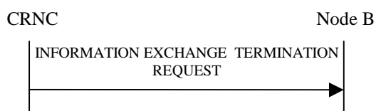
Figure 27O: Information Exchange Termination procedure, Successful Operation
