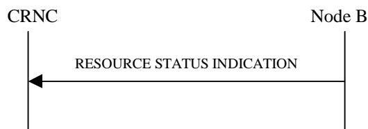
Figure 21: Resource Status Indication procedure, Successful Operation
