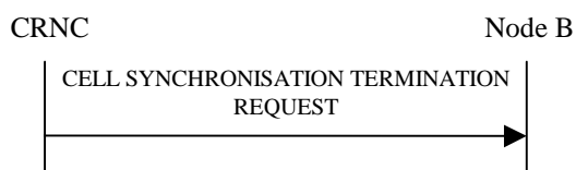
Figure 27H Cell Synchronisation Termination procedure, Successful Operation
