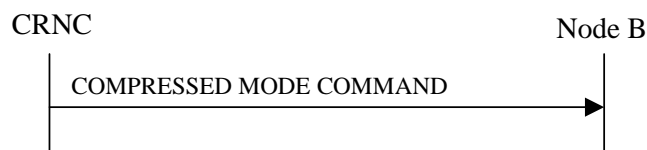
Figure 47: Compressed Mode Command procedure, Successful Operation
