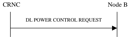
Figure 37: Downlink Power Control procedure, Successful Operation
