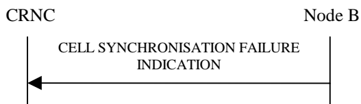
Figure 27I Cell Synchronisation Failure procedure, Successful Operation
