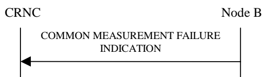
Figure 15: Common Measurement Failure procedure, Successful Operation
