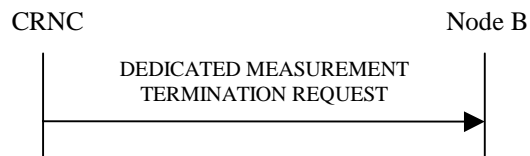
Figure 41: Dedicated Measurement Termination procedure, Successful Operation
