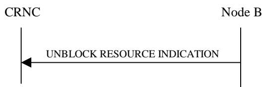
Figure 8: Unblock Resource procedure, Successful Operation
