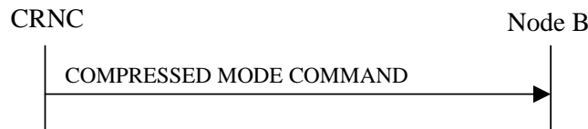
Figure 47: Compressed Mode Command procedure, Successful Operation
