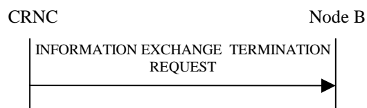
Figure 27O: Information Exchange Termination procedure, Successful Operation
