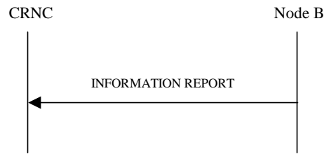
Figure 27N: Information Reporting procedure, Successful Operation
