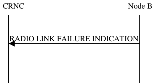
Figure 43: Radio Link Failure procedure, Successful Operation
