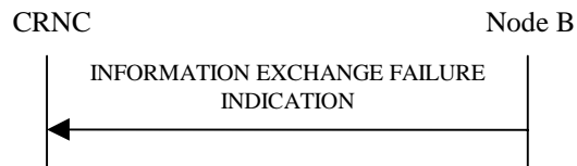
Figure 27P: Information Exchange Failure procedure, Successful Operation
