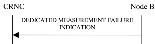
Figure 42: Dedicated Measurement Failure procedure, Successful Operation
