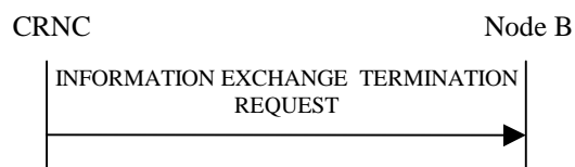
Figure 27O: Information Exchange Termination procedure, Successful Operation
