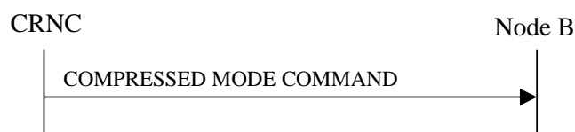
Figure 47: Compressed Mode Command procedure, Successful Operation
