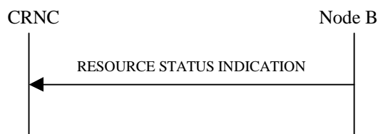
Figure 21: Resource Status Indication procedure, Successful Operation
