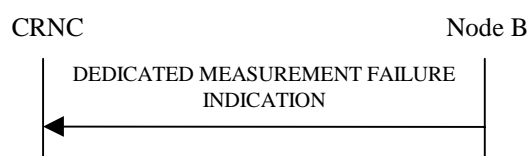
Figure 42: Dedicated Measurement Failure procedure, Successful Operation
