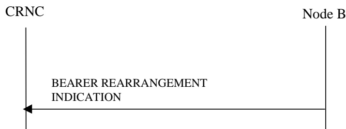
Figure 47C: Bearer Re-arrangement Indication, Successful Operation
