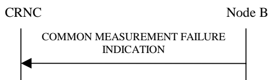
Figure 15: Common Measurement Failure procedure, Successful Operation
