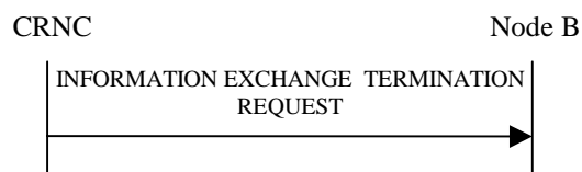
Figure 27O: Information Exchange Termination procedure, Successful Operation
