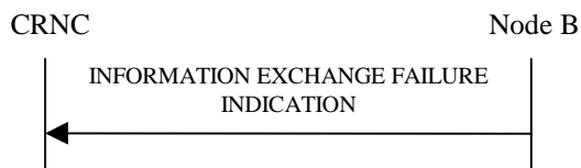
Figure 27P: Information Exchange Failure procedure, Successful Operation
