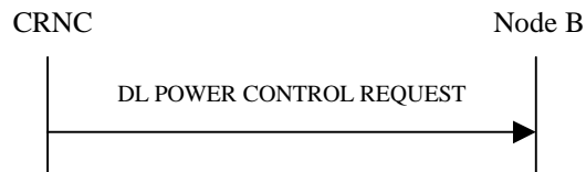
Figure 37: Downlink Power Control procedure, Successful Operation
