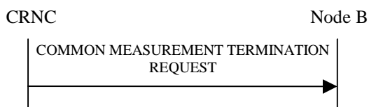
Figure 14: Common Measurement Termination procedure, Successful Operation
