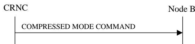
Figure 47: Compressed Mode Command procedure, Successful Operation
