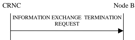
Figure 27O: Information Exchange Termination procedure, Successful Operation
