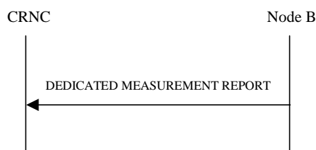
Figure 40: Dedicated Measurement Reporting procedure, Successful Operation
