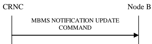
Figure 27Q: MBMS Notification Update procedure, Successful Operation
