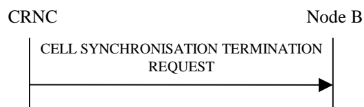
Figure 27H Cell Synchronisation Termination procedure, Successful Operation
