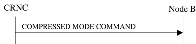
Figure 47: Compressed Mode Command procedure, Successful Operation
