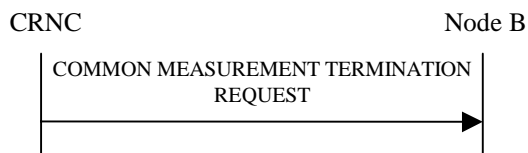
Figure 14: Common Measurement Termination procedure, Successful Operation
