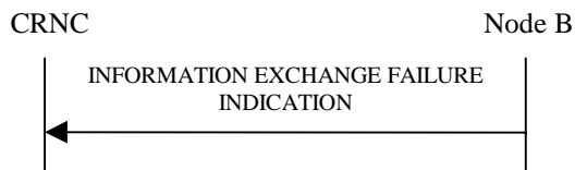
Figure 27P: Information Exchange Failure procedure, Successful Operation
