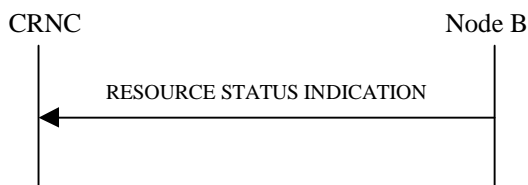
Figure 21: Resource Status Indication procedure, Successful Operation
