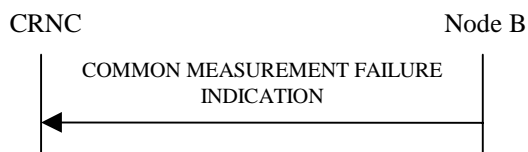
Figure 15: Common Measurement Failure procedure, Successful Operation
