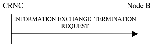
Figure 27O: Information Exchange Termination procedure, Successful Operation
