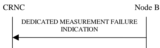
Figure 42: Dedicated Measurement Failure procedure, Successful Operation
