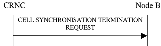
Figure 27H Cell Synchronisation Termination procedure, Successful Operation
