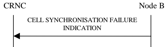
Figure 27I Cell Synchronisation Failure procedure, Successful Operation
