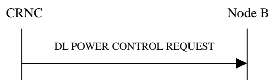
Figure 37: Downlink Power Control procedure, Successful Operation
