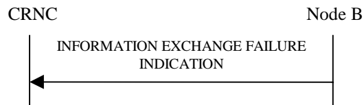
Figure 27P: Information Exchange Failure procedure, Successful Operation
