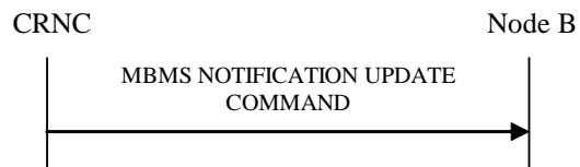
Figure 27Q: MBMS Notification Update procedure, Successful Operation
