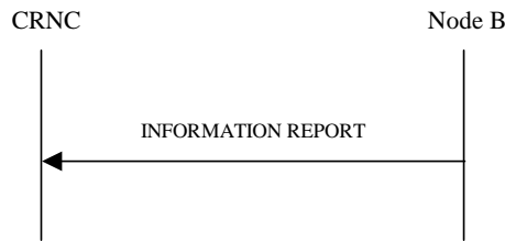
Figure 27N: Information Reporting procedure, Successful Operation
