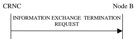
Figure 27O: Information Exchange Termination procedure, Successful Operation
