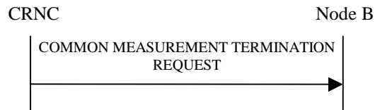
Figure 14: Common Measurement Termination procedure, Successful Operation
