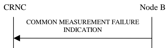
Figure 15: Common Measurement Failure procedure, Successful Operation
