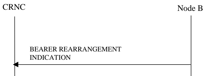
Figure 47C: Bearer Re-arrangement Indication, Successful Operation
