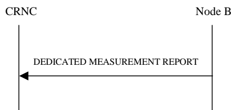
Figure 40: Dedicated Measurement Reporting procedure, Successful Operation
