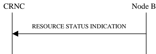
Figure 21: Resource Status Indication procedure, Successful Operation
