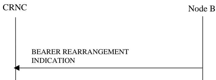
Figure 47C: Bearer Re-arrangement Indication, Successful Operation
