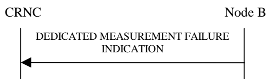
Figure 42: Dedicated Measurement Failure procedure, Successful Operation
