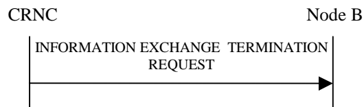
Figure 27O: Information Exchange Termination procedure, Successful Operation
