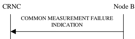
Figure 15: Common Measurement Failure procedure, Successful Operation
