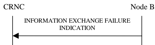
Figure 27P: Information Exchange Failure procedure, Successful Operation
