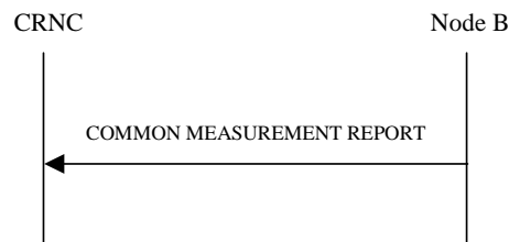
Figure 13: Common Measurement Reporting procedure, Successful Operation
