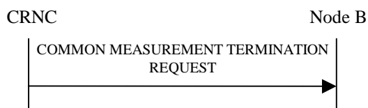
Figure 14: Common Measurement Termination procedure, Successful Operation
