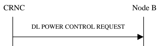
Figure 37: Downlink Power Control procedure, Successful Operation
