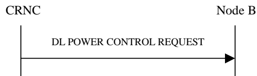
Figure 37: Downlink Power Control procedure, Successful Operation
