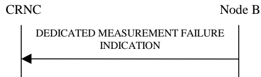
Figure 42: Dedicated Measurement Failure procedure, Successful Operation
