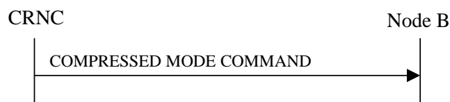
Figure 47: Compressed Mode Command procedure, Successful Operation
