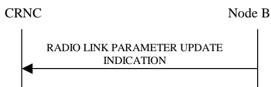
Figure 48: Radio Link Parameter Update Indication, Successful Operation
