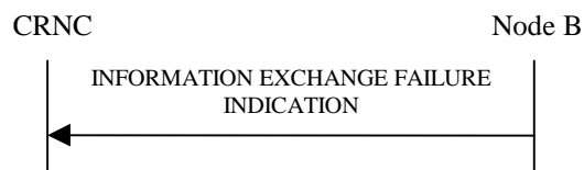
Figure 27P: Information Exchange Failure procedure, Successful Operation
