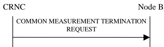
Figure 14: Common Measurement Termination procedure, Successful Operation
