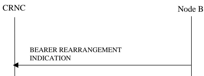
Figure 47C: Bearer Re-arrangement Indication, Successful Operation
