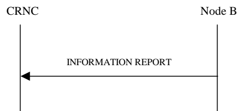
Figure 27N: Information Reporting procedure, Successful Operation
