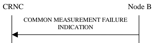
Figure 15: Common Measurement Failure procedure, Successful Operation
