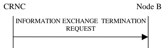
Figure 27O: Information Exchange Termination procedure, Successful Operation
