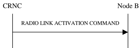
Figure 47D: Radio Link Activation procedure
