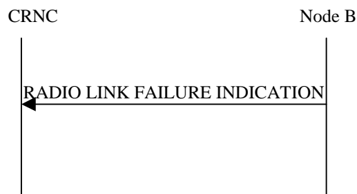
Figure 43: Radio Link Failure procedure, Successful Operation
