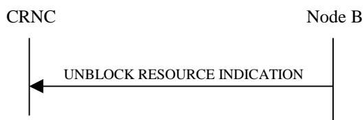
Figure 8: Unblock Resource procedure, Successful Operation
