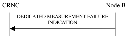
Figure 42: Dedicated Measurement Failure procedure, Successful Operation
