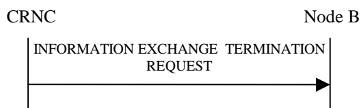
Figure 27O: Information Exchange Termination procedure, Successful Operation
