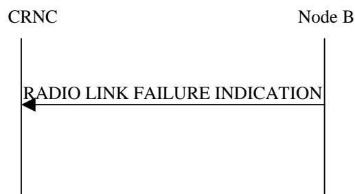
Figure 43: Radio Link Failure procedure, Successful Operation
