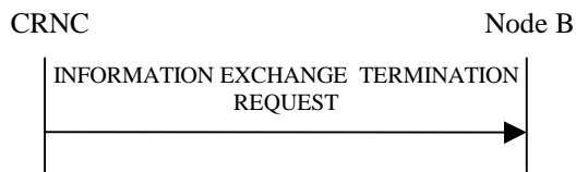
Figure 27O: Information Exchange Termination procedure, Successful Operation
