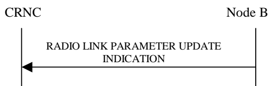
Figure 48: Radio Link Parameter Update Indication, Successful Operation
