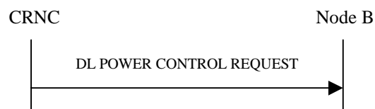
Figure 37: Downlink Power Control procedure, Successful Operation
