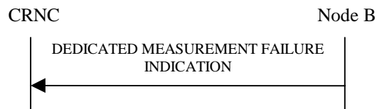
Figure 42: Dedicated Measurement Failure procedure, Successful Operation
