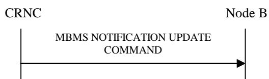
Figure 27Q: MBMS Notification Update procedure, Successful Operation
