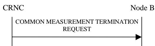
Figure 14: Common Measurement Termination procedure, Successful Operation
