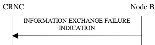
Figure 27P: Information Exchange Failure procedure, Successful Operation
