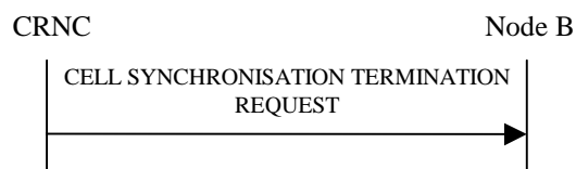
Figure 27H Cell Synchronisation Termination procedure, Successful Operation
