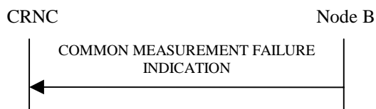
Figure 15: Common Measurement Failure procedure, Successful Operation
