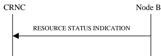
Figure 21: Resource Status Indication procedure, Successful Operation
