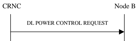
Figure 37: Downlink Power Control procedure, Successful Operation
