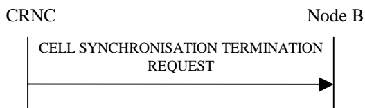
Figure 27H Cell Synchronisation Termination procedure, Successful Operation
