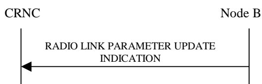
Figure 48: Radio Link Parameter Update Indication, Successful Operation
