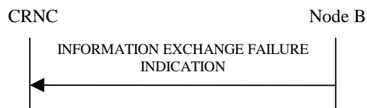
Figure 27P: Information Exchange Failure procedure, Successful Operation
