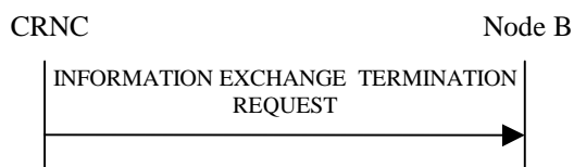
Figure 27O: Information Exchange Termination procedure, Successful Operation
