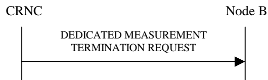
Figure 41: Dedicated Measurement Termination procedure, Successful Operation
