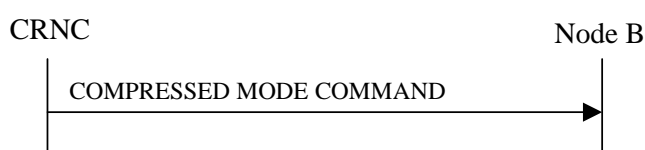
Figure 47: Compressed Mode Command procedure, Successful Operation
