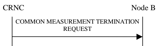
Figure 14: Common Measurement Termination procedure, Successful Operation
