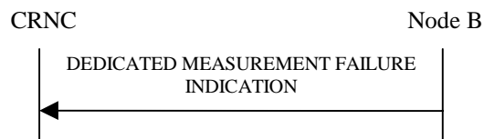
Figure 42: Dedicated Measurement Failure procedure, Successful Operation
