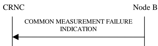
Figure 15: Common Measurement Failure procedure, Successful Operation
