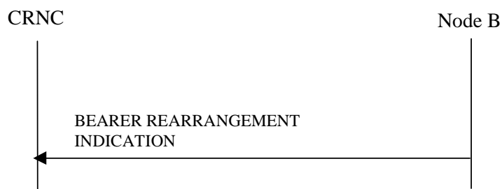
Figure 47C: Bearer Re-arrangement Indication, Successful Operation
