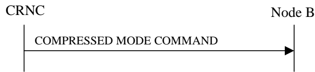
Figure 47: Compressed Mode Command procedure, Successful Operation
