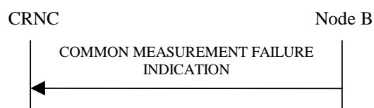
Figure 15: Common Measurement Failure procedure, Successful Operation
