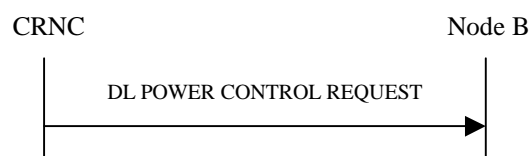
Figure 37: Downlink Power Control procedure, Successful Operation
