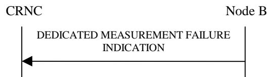
Figure 42: Dedicated Measurement Failure procedure, Successful Operation
