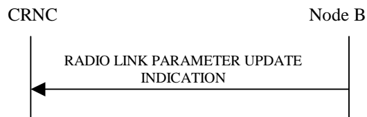
Figure 48: Radio Link Parameter Update Indication, Successful Operation
