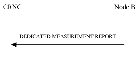
Figure 40: Dedicated Measurement Reporting procedure, Successful Operation
