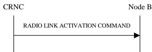
Figure 47D: Radio Link Activation procedure
