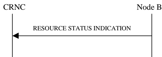
Figure 21: Resource Status Indication procedure, Successful Operation
