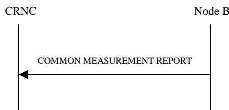
Figure 13: Common Measurement Reporting procedure, Successful Operation
