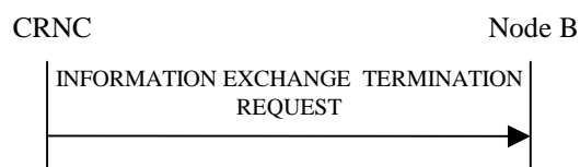
Figure 27O: Information Exchange Termination procedure, Successful Operation
