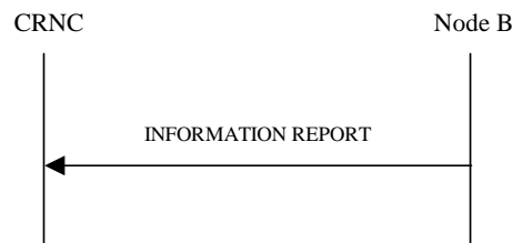
Figure 27N: Information Reporting procedure, Successful Operation
