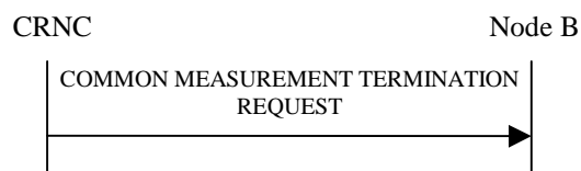
Figure 14: Common Measurement Termination procedure, Successful Operation
