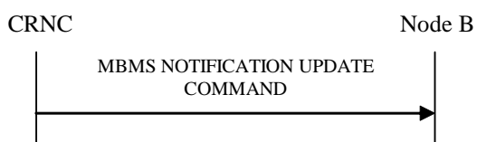
Figure 27Q: MBMS Notification Update procedure, Successful Operation
