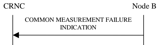
Figure 15: Common Measurement Failure procedure, Successful Operation
