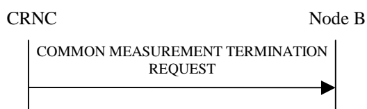
Figure 14: Common Measurement Termination procedure, Successful Operation
