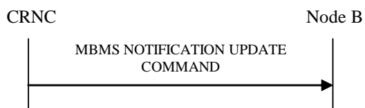
Figure 27Q: MBMS Notification Update procedure, Successful Operation
