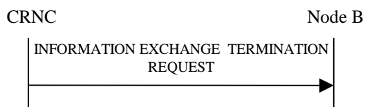
Figure 27O: Information Exchange Termination procedure, Successful Operation
