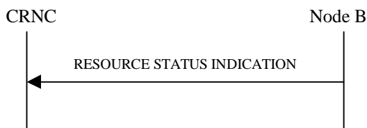
Figure 21: Resource Status Indication procedure, Successful Operation
