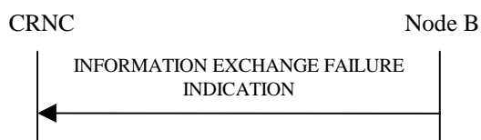
Figure 27P: Information Exchange Failure procedure, Successful Operation
