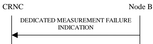
Figure 42: Dedicated Measurement Failure procedure, Successful Operation
