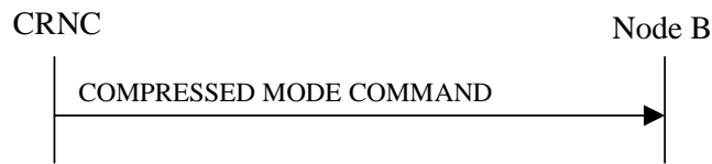
Figure 47: Compressed Mode Command procedure, Successful Operation
