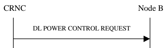
Figure 37: Downlink Power Control procedure, Successful Operation
