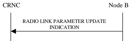
Figure 48: Radio Link Parameter Update Indication, Successful Operation
