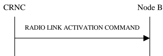
Figure 47D: Radio Link Activation procedure
