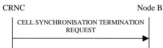
Figure 27H Cell Synchronisation Termination procedure, Successful Operation
