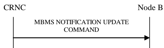
Figure 27Q: MBMS Notification Update procedure, Successful Operation
