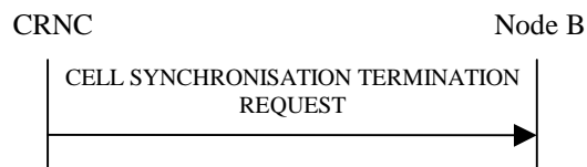
Figure 27H Cell Synchronisation Termination procedure, Successful Operation
