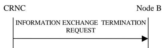
Figure 27O: Information Exchange Termination procedure, Successful Operation
