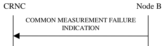
Figure 15: Common Measurement Failure procedure, Successful Operation
