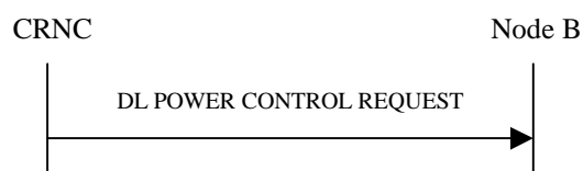
Figure 37: Downlink Power Control procedure, Successful Operation
