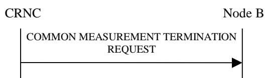
Figure 14: Common Measurement Termination procedure, Successful Operation
