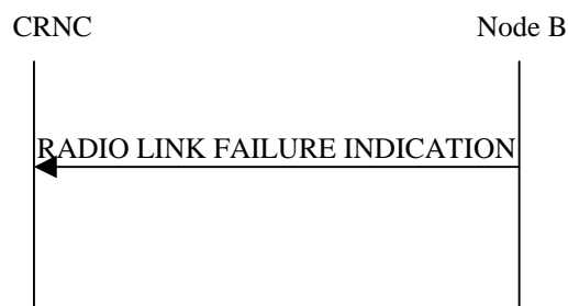
Figure 43: Radio Link Failure procedure, Successful Operation
