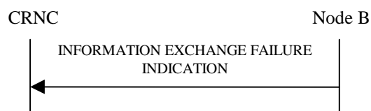
Figure 27P: Information Exchange Failure procedure, Successful Operation
