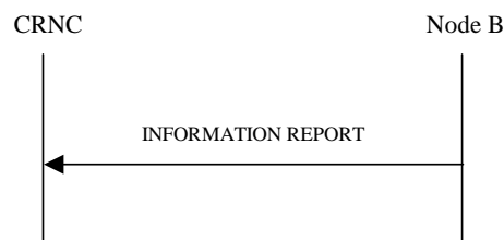
Figure 27N: Information Reporting procedure, Successful Operation
