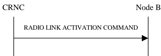
Figure 47D: Radio Link Activation procedure
