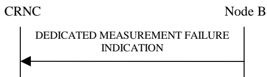
Figure 42: Dedicated Measurement Failure procedure, Successful Operation
