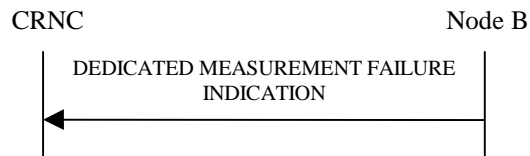
Figure 42: Dedicated Measurement Failure procedure, Successful Operation
