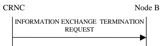
Figure 27O: Information Exchange Termination procedure, Successful Operation
