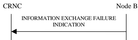
Figure 27P: Information Exchange Failure procedure, Successful Operation
