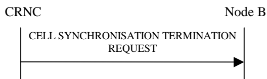
Figure 27H Cell Synchronisation Termination procedure, Successful Operation
