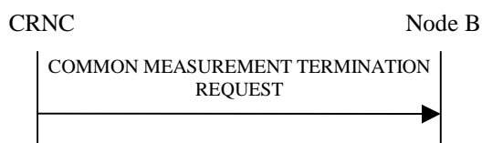
Figure 14: Common Measurement Termination procedure, Successful Operation
