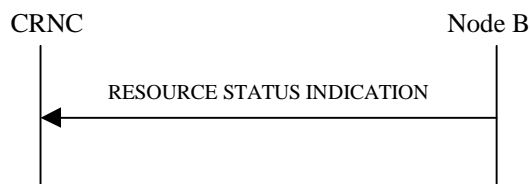
Figure 21: Resource Status Indication procedure, Successful Operation
