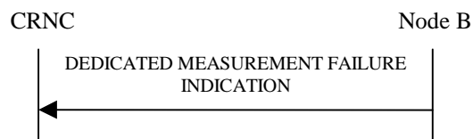
Figure 42: Dedicated Measurement Failure procedure, Successful Operation
