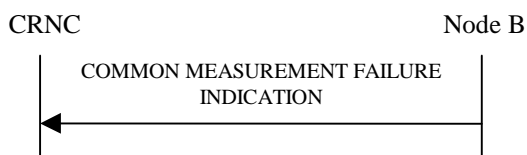
Figure 15: Common Measurement Failure procedure, Successful Operation
