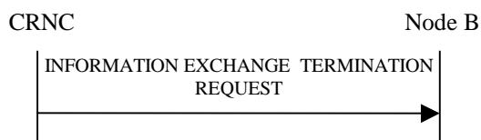
Figure 27O: Information Exchange Termination procedure, Successful Operation
