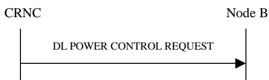
Figure 37: Downlink Power Control procedure, Successful Operation
