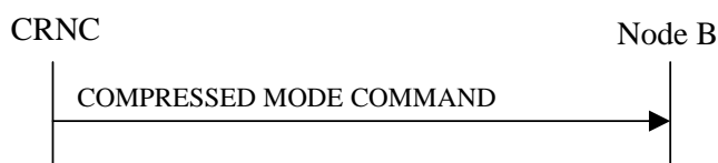
Figure 47: Compressed Mode Command procedure, Successful Operation
