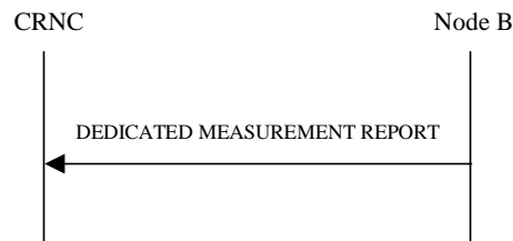
Figure 40: Dedicated Measurement Reporting procedure, Successful Operation
