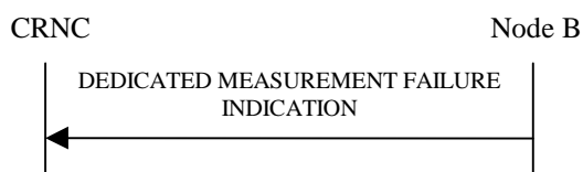
Figure 42: Dedicated Measurement Failure procedure, Successful Operation
