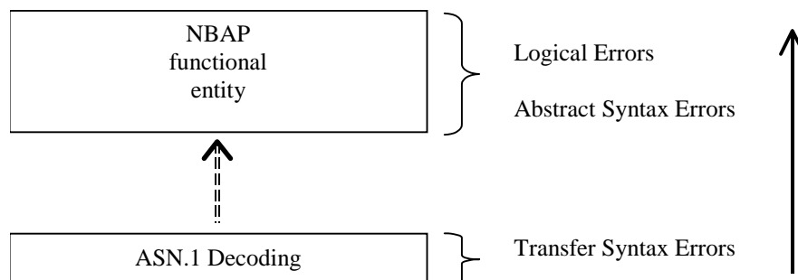
Figure 38: Protocol Errors in NBAP.
