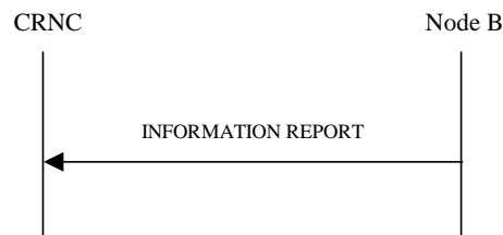
Figure 27N: Information Reporting procedure, Successful Operation
