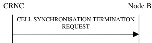
Figure 27H Cell Synchronisation Termination procedure, Successful Operation
