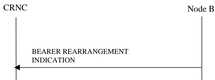
Figure 47C: Bearer Re-arrangement Indication, Successful Operation
