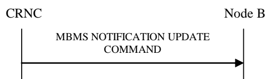
Figure 27Q: MBMS Notification Update procedure, Successful Operation
