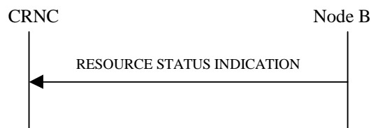
Figure 21: Resource Status Indication procedure, Successful Operation
