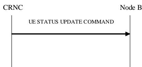
Figure 27R: UE Status Update procedure, Successful Operation
