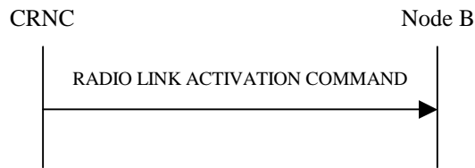
Figure 47D: Radio Link Activation procedure
