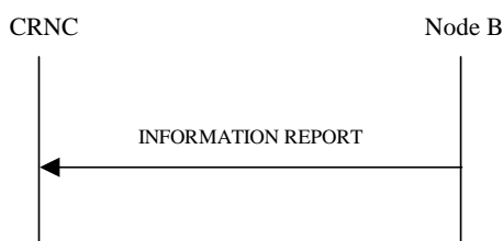
Figure 27N: Information Reporting procedure, Successful Operation
