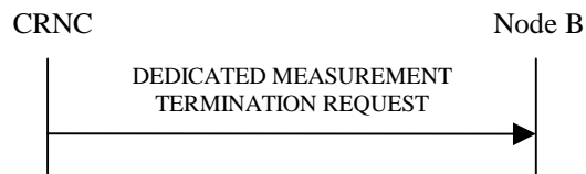
Figure 41: Dedicated Measurement Termination procedure, Successful Operation
