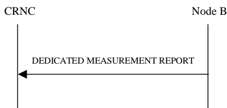
Figure 40: Dedicated Measurement Reporting procedure, Successful Operation
