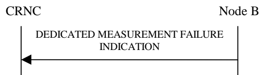
Figure 42: Dedicated Measurement Failure procedure, Successful Operation
