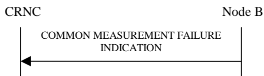
Figure 15: Common Measurement Failure procedure, Successful Operation
