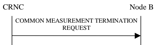
Figure 14: Common Measurement Termination procedure, Successful Operation
