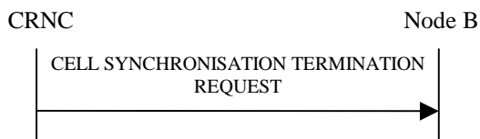
Figure 27H Cell Synchronisation Termination procedure, Successful Operation
