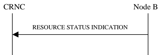
Figure 21: Resource Status Indication procedure, Successful Operation
