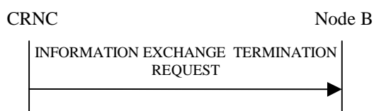
Figure 27O: Information Exchange Termination procedure, Successful Operation
