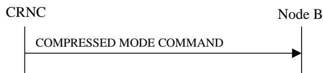
Figure 47: Compressed Mode Command procedure, Successful Operation
