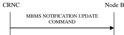
Figure 27Q: MBMS Notification Update procedure, Successful Operation
