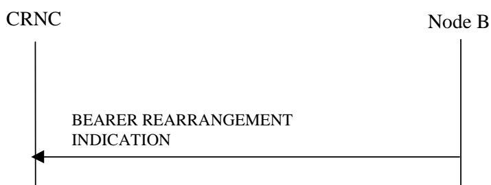
Figure 47C: Bearer Re-arrangement Indication, Successful Operation
