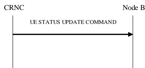
Figure 27R: UE Status Update procedure, Successful Operation
