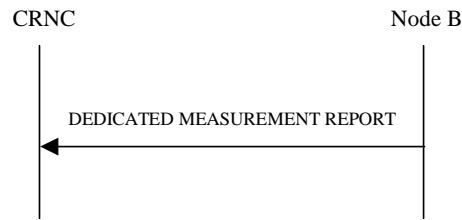
Figure 40: Dedicated Measurement Reporting procedure, Successful Operation
