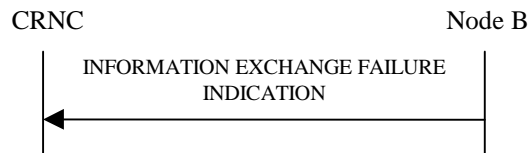
Figure 27P: Information Exchange Failure procedure, Successful Operation
