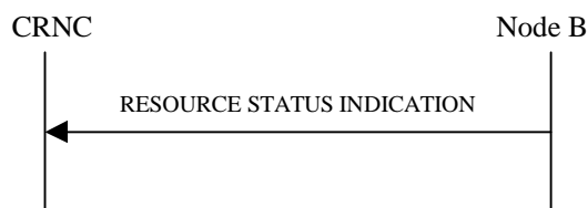
Figure 21: Resource Status Indication procedure, Successful Operation
