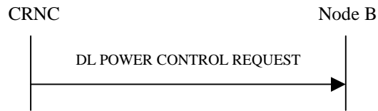
Figure 37: Downlink Power Control procedure, Successful Operation
