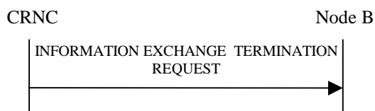
Figure 27O: Information Exchange Termination procedure, Successful Operation
