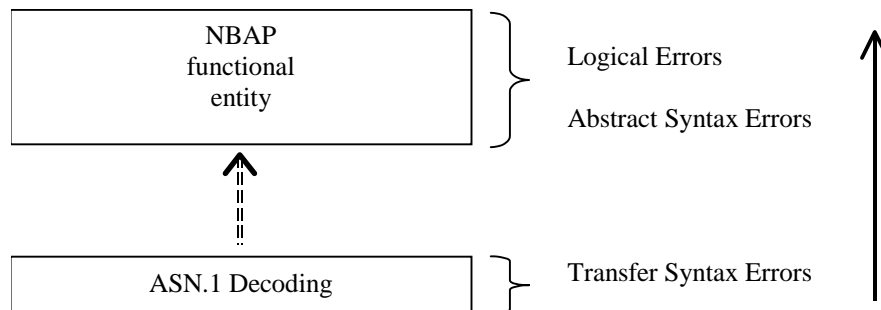
Figure 38: Protocol Errors in NBAP.
