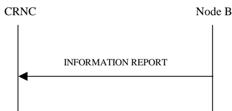
Figure 27N: Information Reporting procedure, Successful Operation
