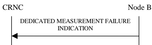
Figure 42: Dedicated Measurement Failure procedure, Successful Operation
