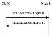
Figure 20: Cell Deletion procedure, Successful Operation
