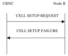
Figure 17: Cell Setup procedure: Unsuccessful Operation
