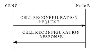
Figure 18: Cell Reconfiguration procedure, Successful Operation
