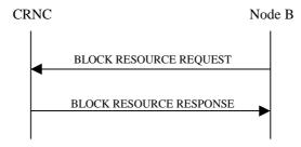
Figure 6: Block Resource procedure, Successful Operation
