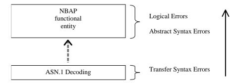
Figure 38: Protocol Errors in NBAP.
