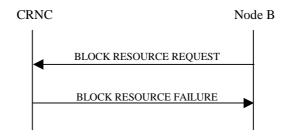
Figure 7: Block Resource procedure, Unsuccessful Operation
