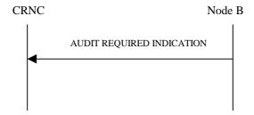
Figure 9: Audit Required procedure, Successful Operation
