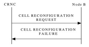
Figure 19: Cell Reconfiguration procedure: Unsuccessful Operation
