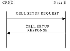
Figure 16: Cell Setup procedure, Successful Operation
