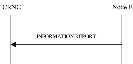
Figure 27N: Information Reporting procedure, Successful Operation
