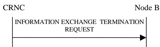
Figure 27O: Information Exchange Termination procedure, Successful Operation
