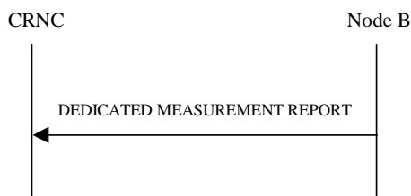
Figure 40: Dedicated Measurement Reporting procedure, Successful Operation
