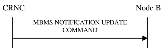
Figure 27Q: MBMS Notification Update procedure, Successful Operation
