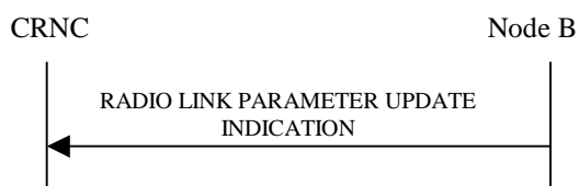
Figure 48: Radio Link Parameter Update Indication, Successful Operation
