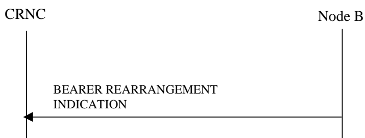
Figure 47C: Bearer Re-arrangement Indication, Successful Operation
