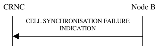
Figure 27I Cell Synchronisation Failure procedure, Successful Operation
