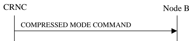
Figure 47: Compressed Mode Command procedure, Successful Operation
