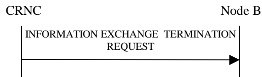
Figure 27O: Information Exchange Termination procedure, Successful Operation
