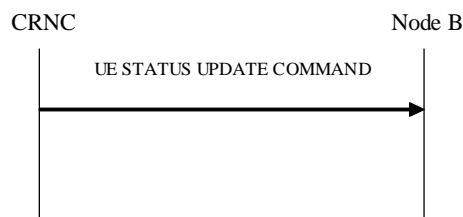
Figure 27R: UE Status Update procedure, Successful Operation
