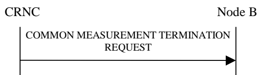
Figure 14: Common Measurement Termination procedure, Successful Operation
