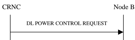
Figure 37: Downlink Power Control procedure, Successful Operation
