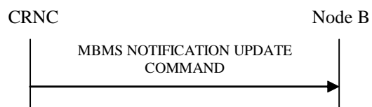
Figure 27Q: MBMS Notification Update procedure, Successful Operation
