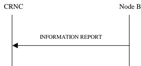
Figure 27N: Information Reporting procedure, Successful Operation
