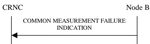
Figure 15: Common Measurement Failure procedure, Successful Operation
