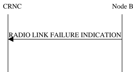
Figure 43: Radio Link Failure procedure, Successful Operation
