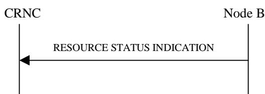
Figure 21: Resource Status Indication procedure, Successful Operation
