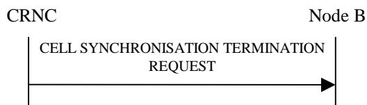
Figure 27H Cell Synchronisation Termination procedure, Successful Operation
