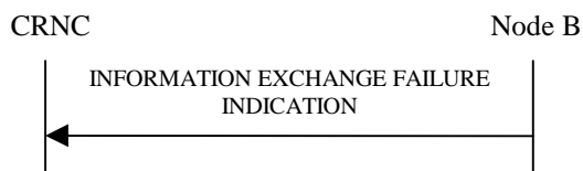
Figure 27P: Information Exchange Failure procedure, Successful Operation
