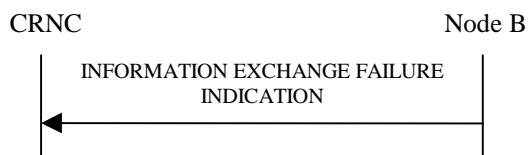
Figure 27P: Information Exchange Failure procedure, Successful Operation
