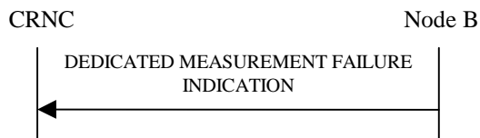
Figure 42: Dedicated Measurement Failure procedure, Successful Operation
