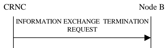
Figure 27O: Information Exchange Termination procedure, Successful Operation
