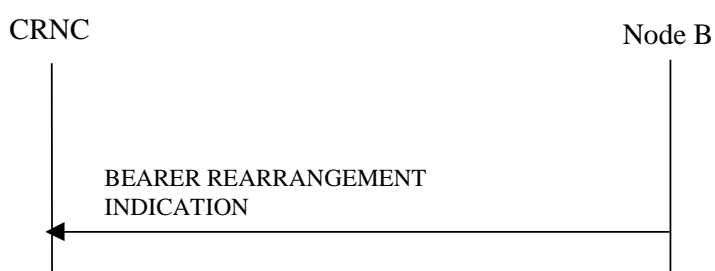
Figure 47C: Bearer Re-arrangement Indication, Successful Operation
