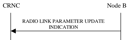
Figure 48: Radio Link Parameter Update Indication, Successful Operation
