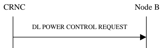
Figure 37: Downlink Power Control procedure, Successful Operation
