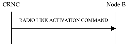
Figure 47D: Radio Link Activation procedure
