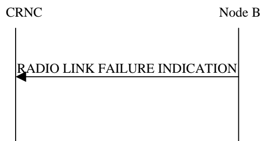
Figure 43: Radio Link Failure procedure, Successful Operation
