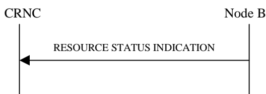
Figure 21: Resource Status Indication procedure, Successful Operation
