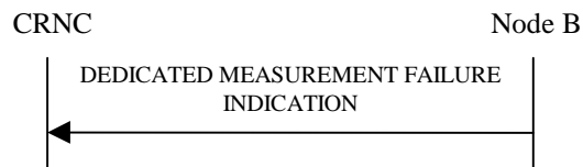
Figure 42: Dedicated Measurement Failure procedure, Successful Operation
