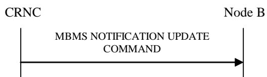
Figure 27Q: MBMS Notification Update procedure, Successful Operation
