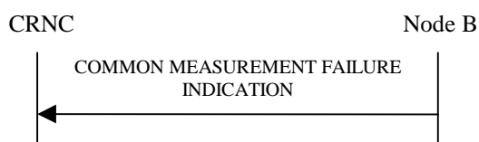
Figure 15: Common Measurement Failure procedure, Successful Operation
