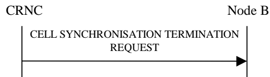
Figure 27H Cell Synchronisation Termination procedure, Successful Operation
