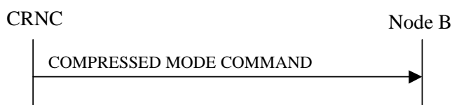
Figure 47: Compressed Mode Command procedure, Successful Operation
