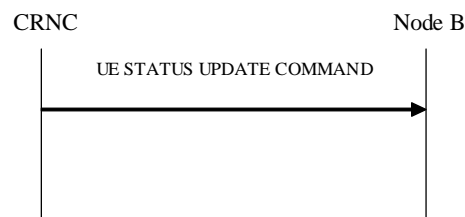
Figure 27R: UE Status Update procedure, Successful Operation
