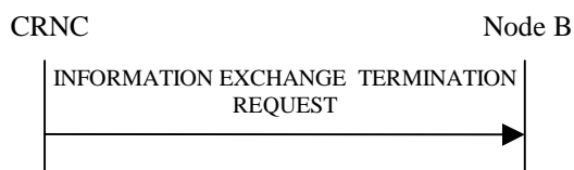
Figure 27O: Information Exchange Termination procedure, Successful Operation
