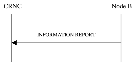
Figure 27N: Information Reporting procedure, Successful Operation
