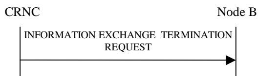
Figure 27O: Information Exchange Termination procedure, Successful Operation
