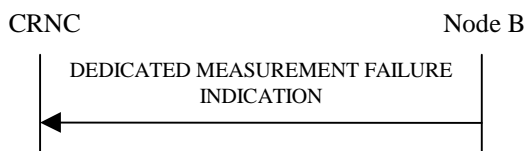
Figure 42: Dedicated Measurement Failure procedure, Successful Operation
