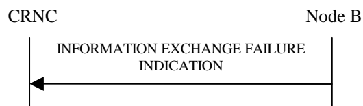
Figure 27P: Information Exchange Failure procedure, Successful Operation
