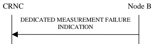
Figure 42: Dedicated Measurement Failure procedure, Successful Operation
