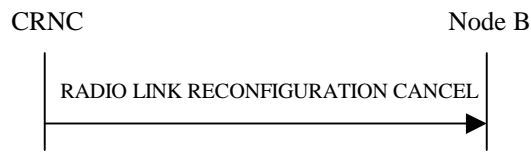
Figure 33: Synchronised Radio Link Reconfiguration Cancellation procedure, Successful Operation
