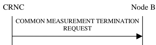
Figure 14: Common Measurement Termination procedure, Successful Operation
