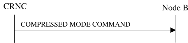
Figure 47: Compressed Mode Command procedure, Successful Operation
