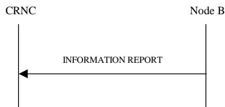
Figure 27N: Information Reporting procedure, Successful Operation
