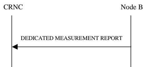
Figure 40: Dedicated Measurement Reporting procedure, Successful Operation
