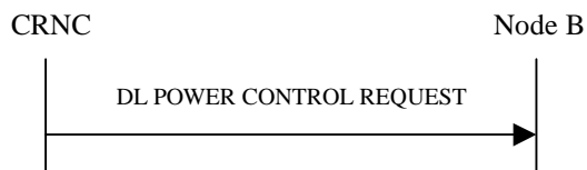
Figure 37: Downlink Power Control procedure, Successful Operation
