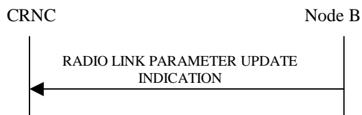
Figure 48: Radio Link Parameter Update Indication, Successful Operation
