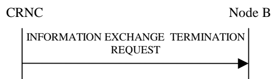
Figure 27O: Information Exchange Termination procedure, Successful Operation
