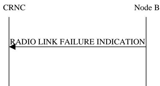
Figure 43: Radio Link Failure procedure, Successful Operation
