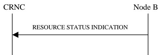
Figure 21: Resource Status Indication procedure, Successful Operation
