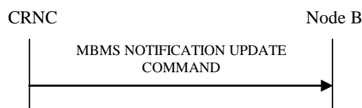
Figure 27Q: MBMS Notification Update procedure, Successful Operation
