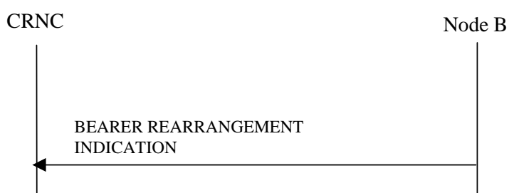
Figure 47C: Bearer Re-arrangement Indication, Successful Operation
