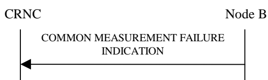
Figure 15: Common Measurement Failure procedure, Successful Operation
