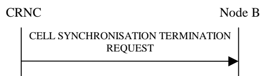
Figure 27H Cell Synchronisation Termination procedure, Successful Operation
