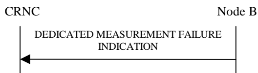
Figure 42: Dedicated Measurement Failure procedure, Successful Operation
