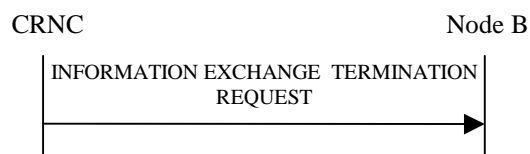
Figure 27O: Information Exchange Termination procedure, Successful Operation
