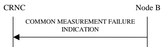
Figure 15: Common Measurement Failure procedure, Successful Operation
