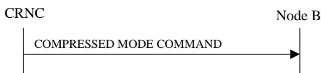
Figure 47: Compressed Mode Command procedure, Successful Operation
