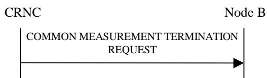
Figure 14: Common Measurement Termination procedure, Successful Operation
