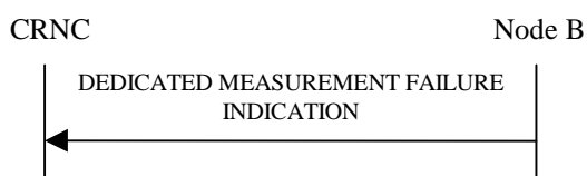
Figure 42: Dedicated Measurement Failure procedure, Successful Operation
