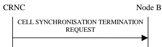
Figure 27H Cell Synchronisation Termination procedure, Successful Operation
