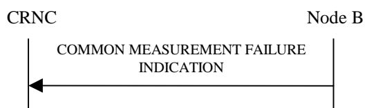
Figure 15: Common Measurement Failure procedure, Successful Operation
