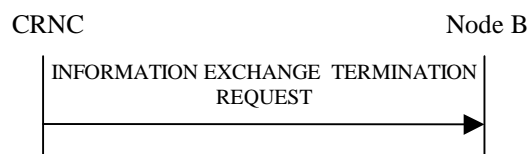
Figure 27O: Information Exchange Termination procedure, Successful Operation
