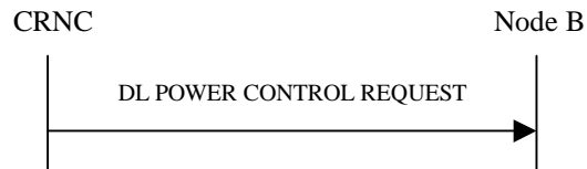
Figure 37: Downlink Power Control procedure, Successful Operation
