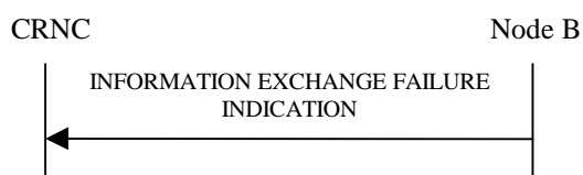
Figure 27P: Information Exchange Failure procedure, Successful Operation
