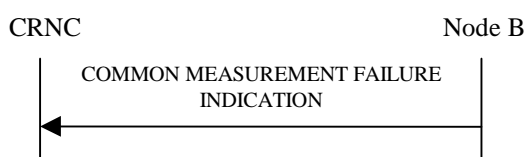
Figure 15: Common Measurement Failure procedure, Successful Operation
