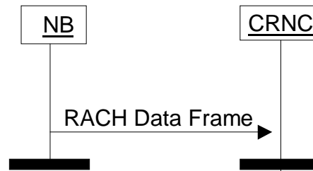
Figure 1: RACH Data Transfer Procedure
