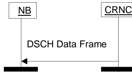
Figure 5: DSCH Data Transfer Procedure
