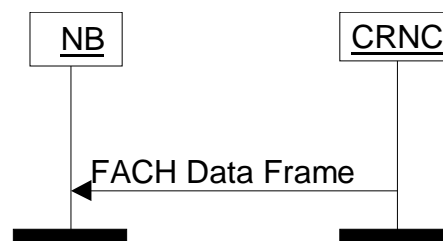
Figure 3: FACH Data Transfer Procedure
