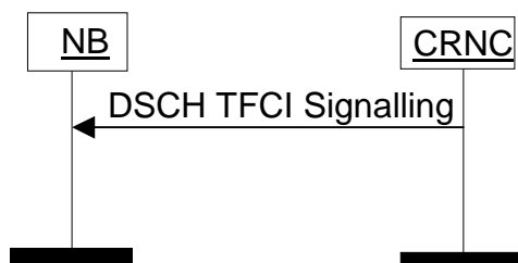
Figure 11: DSCH TFCI Signalling
